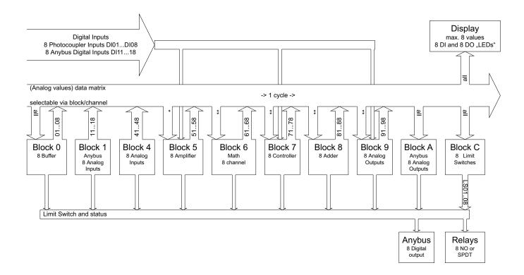
Up to 8 analog values from the data matrix can be displayed. All block outputs are scheduled as a source. This simplifies troubleshooting in customer systems, eg. the raw data of the sensor signals can be checked without a measuring device.
