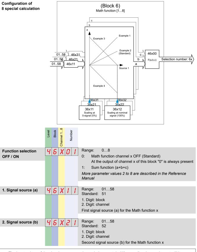
The input values of the signal sources can be scaled separately. When scaling the result must still be within the permitted range. The result will be limited to  $\pm 200\%$ . A Tabular overview of signal sources is given in chapter 8
