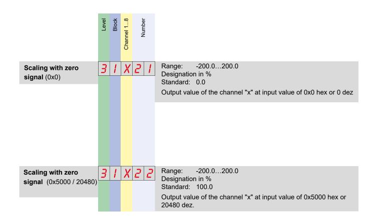
The input values of the signal sources can be scaled separately. When scaling the result must still be within the permitted range. The result will be limited to  $\pm$  200%. Sample calculations for scaling can be found in chapter 6.3.3.
