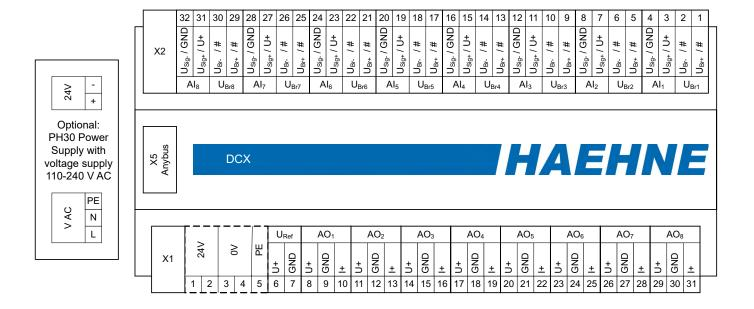
With the optional power supply of 110-240 V AC and the housings G1 to G4, the 24 V supply is pre-wired for the power supply PH30 (X1: terminal 1 and 3).
