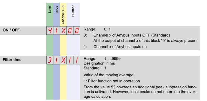
Within the individual blocks of the DCX more filter functions are selectable, in addition to the input filters. The combination of these functions results in a total filter effect.
