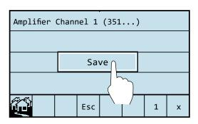
By pressing the "Save" field the changed parameter values of the amplifier channel (Level / Block / Channel) are stored in the long term memory.
