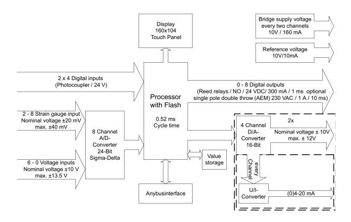
The DCX is a user-oriented combination of functional units which are arranged around the core: the Digital Signal Processor. This runs synchronously to the A / D converter with a cycle time of 0.52 ms. In one clock cycle every eight converter signals, present in the A / D, are read, processed and issued again with 16 bit resolution.
