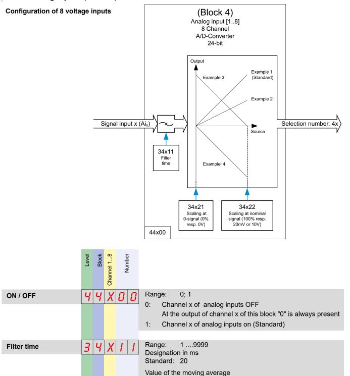
$\frac{O}{I}$  Within the individual blocks of the DCX more filter functions are selectable, in addition to the input filters. The combination of these functions results in a total filter effect.
