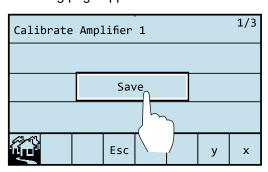
By pressing "Save" the changed parameter values are transferred to the long-term memory. In contrast, the page is exited by pressing "Esc" without saving the entries.
