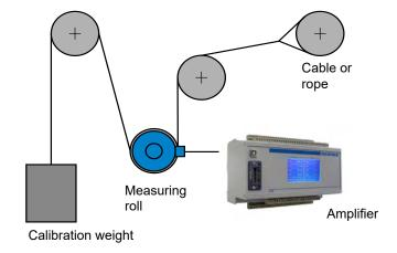
9. Under parameter 35x21 (s. chapter 4.2.4. Adjustment Mode) the percent value of the reference weight in relation to the maximum force. Use the "Quick Function for adjusting the amplification" (refer to 4.2.3 Quick Functions). After adjustment a voltage is available at the amplifier output which is proportional to the percent value. In case of 100 % of the utilized maximum force the voltage is 10 V.
